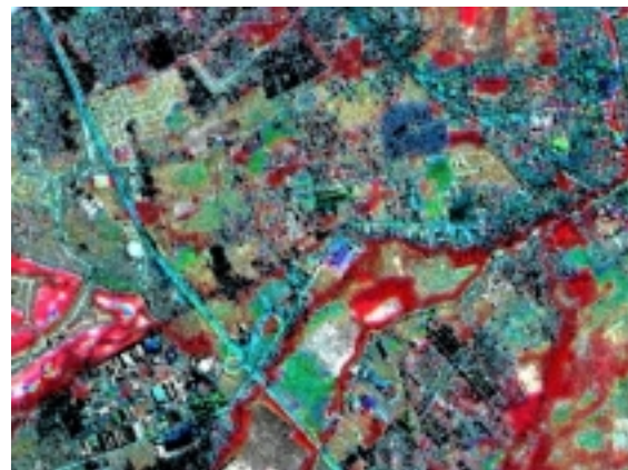
Figure 4b. RGB Combination of SPOT XS and NASA-JPL POLSAR - Cvv of Carmona and Biñan, showing more spectral detail and spatial enhancements. Built-up areas are highlighted in blue and dark areas, while vegetation appear in red and green.
